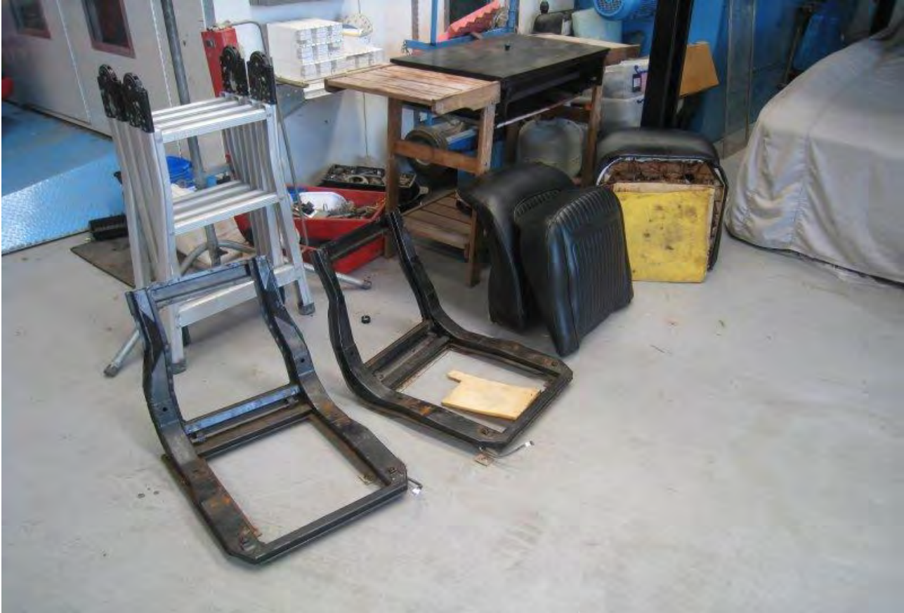
First steps were to remove the bonnet and seats, and connections to the dash plate.
