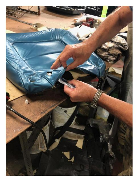
He removed the cover off the foam and glued a mesh "back" to the underside of the seat cover.
