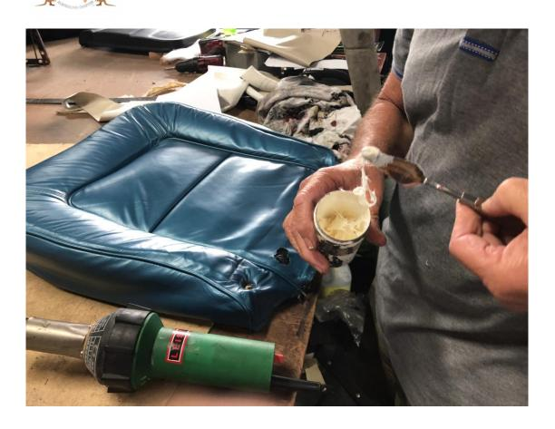
He then, with a spatula, applied vinyl paste with a fibrous filling in it, then, used the heat gun to set it.
