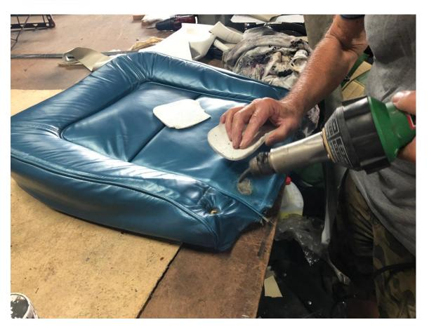
He did this process twice and then a third covering of just the straight vinyl paste. Just before he set it with the heat gun, he pressed a piece of leather into it to give it a leather grain and then set it with the heat gun.
