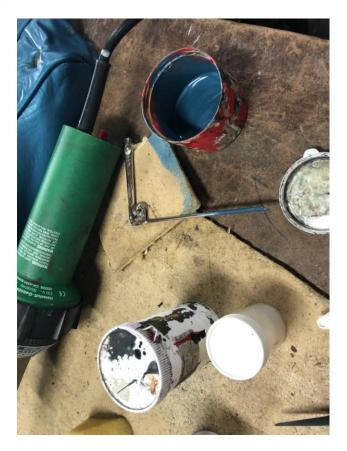
Once he had finished the process, he then mixed up dye to match the seat and applied it with a small mouth blown spray gun, which gave him the right colour but a flat finish.
