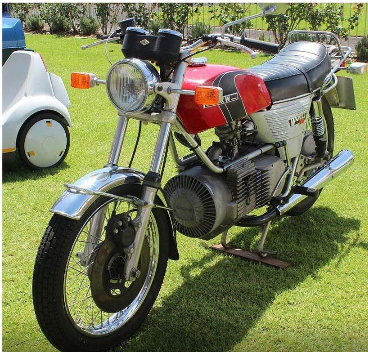
The Hercules W-2000 was a motorcycle made by Hercules in Germany. It was the first production motorcycle with a Wankel engine. Only 1800 were manufactured.
