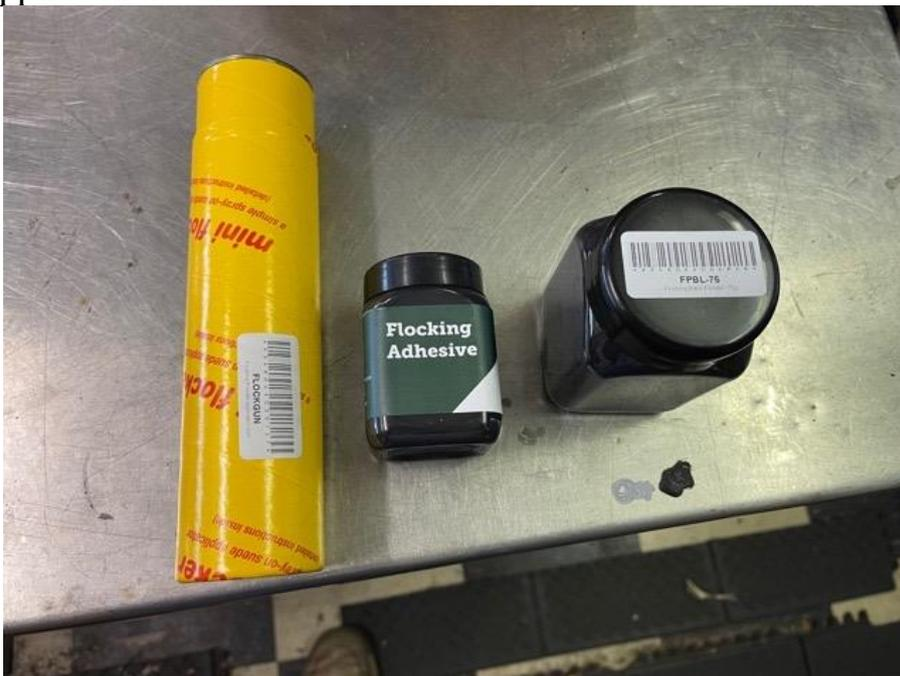
If you hop onto the internet and type in Flocking Powder Repair Kit, you will be able to find the supplier. The yellow hand pump, the flocking agent and the adhesive
