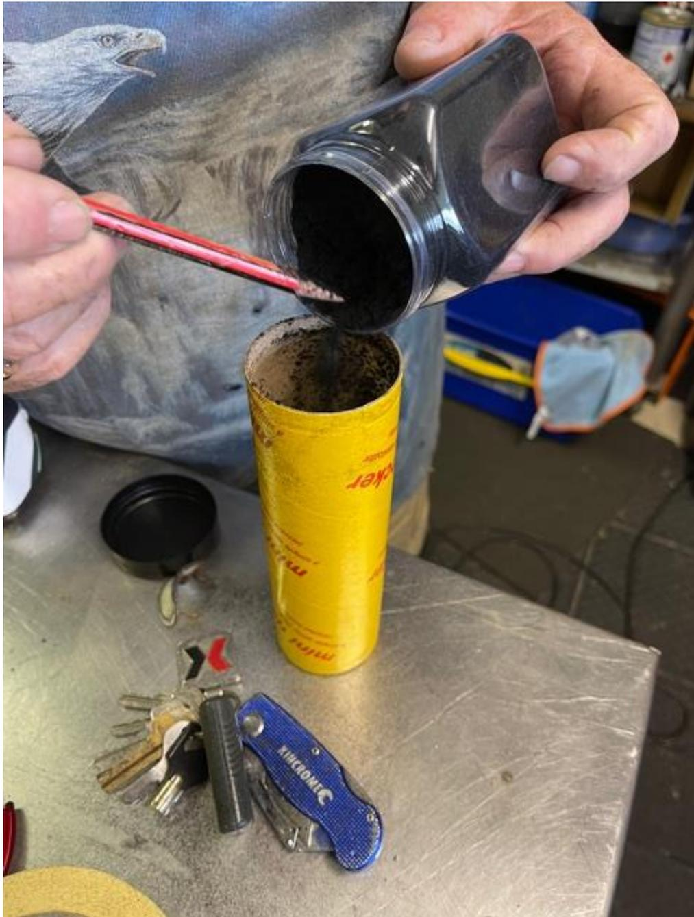
Filling the hand pump with the flocking agent, the pump works by another section that slips in the outside section. It then has a series of holes in its end, which you then hold the outer section and pump the inner section in and out which then sprays the flock powder over the adhesive you have painted on.
