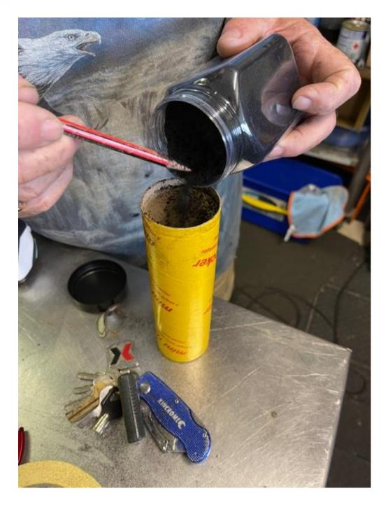
Filling the hand pump with the flocking agent, the pump works by another section that slips In the outside section. It then has a series of holes in its end, which you then hold the Outer section and pump the inner section in and out which then sprays the flock powder Over the adhesive you have painted on.
