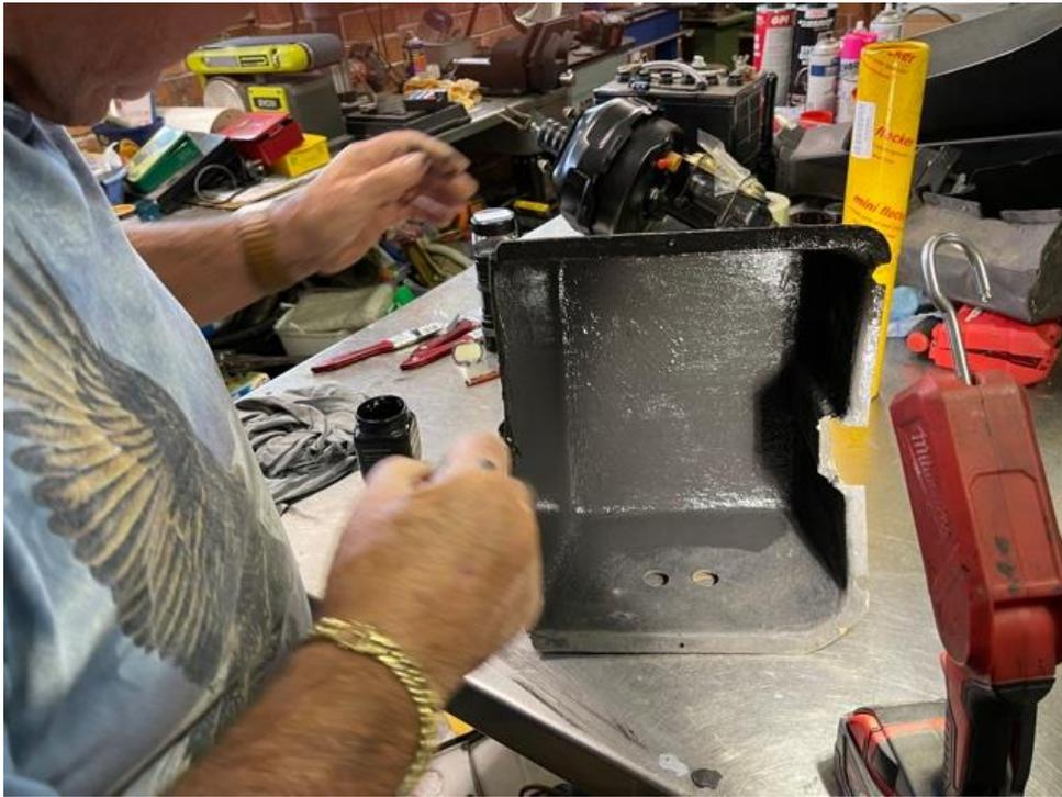
Painting on the adhesive above and pumping the flocking powder onto the compartment
