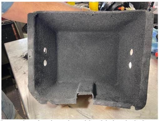
Leave it for a couple of hours to dry and you have reinstated the original coating back onto the units.
