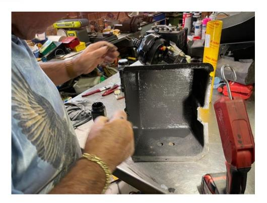
Painting on the adhesive above and pumping the flocking powder onto the compartment Once you have covered the whole area, turn the unit upside down onto a clean surface and tap it, all the excess flocking agent will fall out which you then can put it back into its own container to be re-used for the next time
