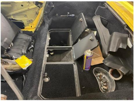
I am working on a restoration of a 69 C3 and after speaking to Terry Martin, he told me About a product called Flocking. It is a process where you paint on an adhesive, fill a pump Container with very fine flocking powder. You then pump on the powder using the hand
