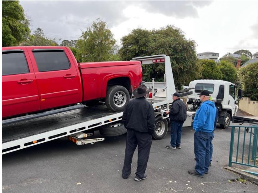
Unfortunately, the truck with all the bags decided to break down. It blew the top out of the steering box, which caused me to lose power steering and power brakes. We then flat towed it to Hobart to have the repairs carried out.
