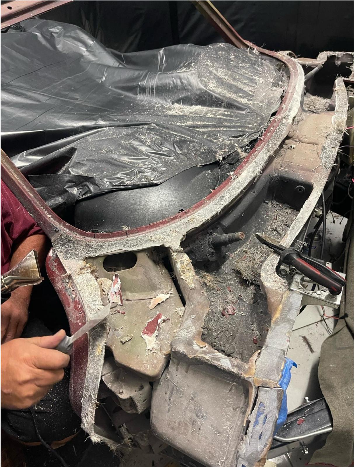
We uncovered previous damage to the heater box area, which we had to repair before we could install the new clip.
