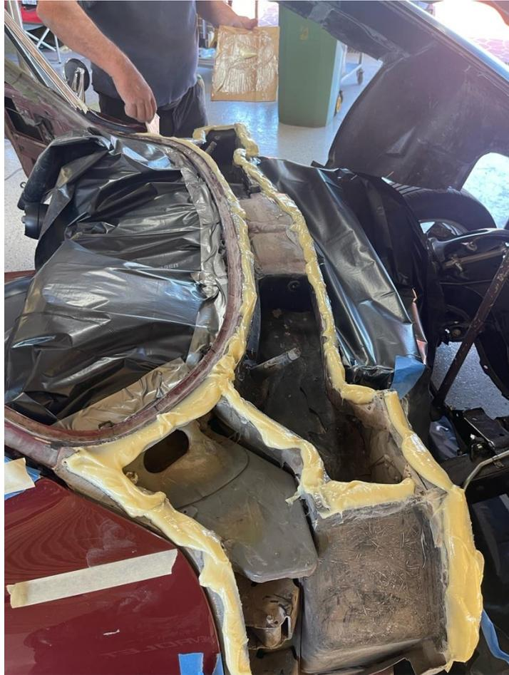
After we had done a trial with the front clip, we then mixed up and installed the bonding agent.
