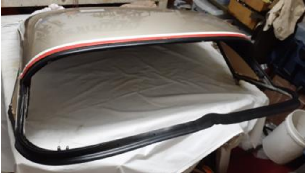
Figure 3. New rubber for the rear windows is all one piece, including side windows. Here with new side windows in. Protective tape to avoid slipping and scratching the top.
