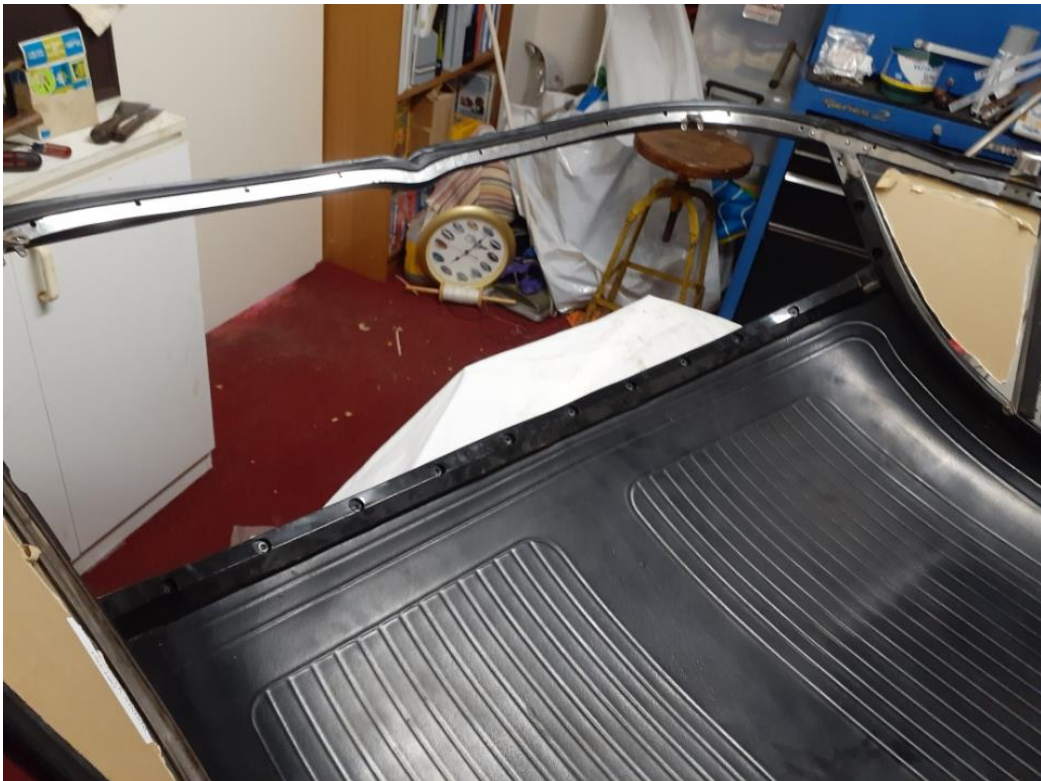
Figure 4. The holes in the new rubbers do not match any of the holes in the frames surrounding the side and rear windows. New rubbers had to be drilled to match frames.
