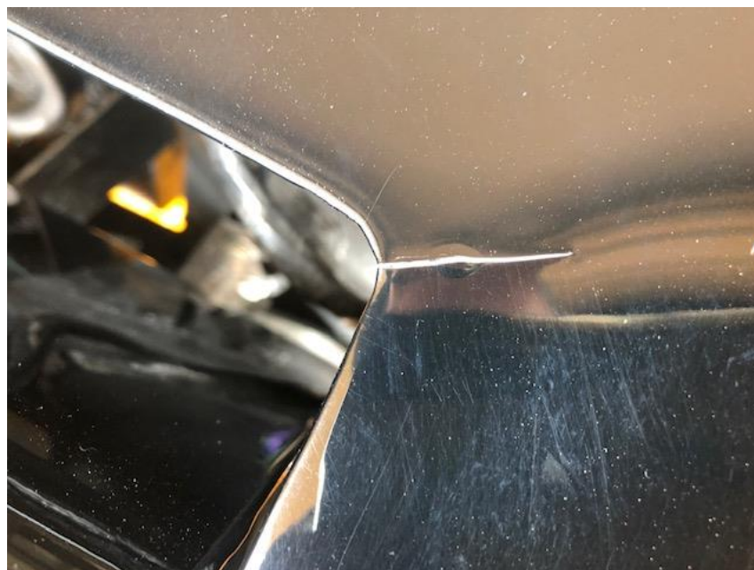
Also cracks on corners of both front headlight buckets
