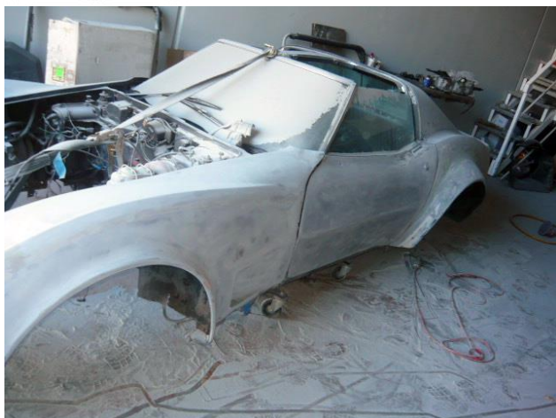
Paint removal and note top of front fender coming away from the birdcage.
