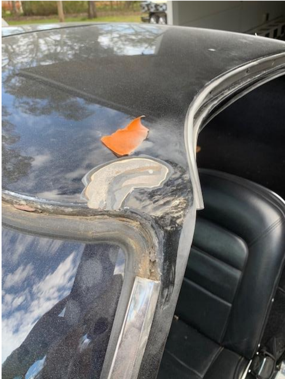
Cracked above drivers' side front windscreen.
