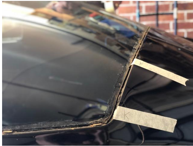
Note the cracks at base of windows
