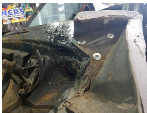
Bonding strip to birdcage repair.
