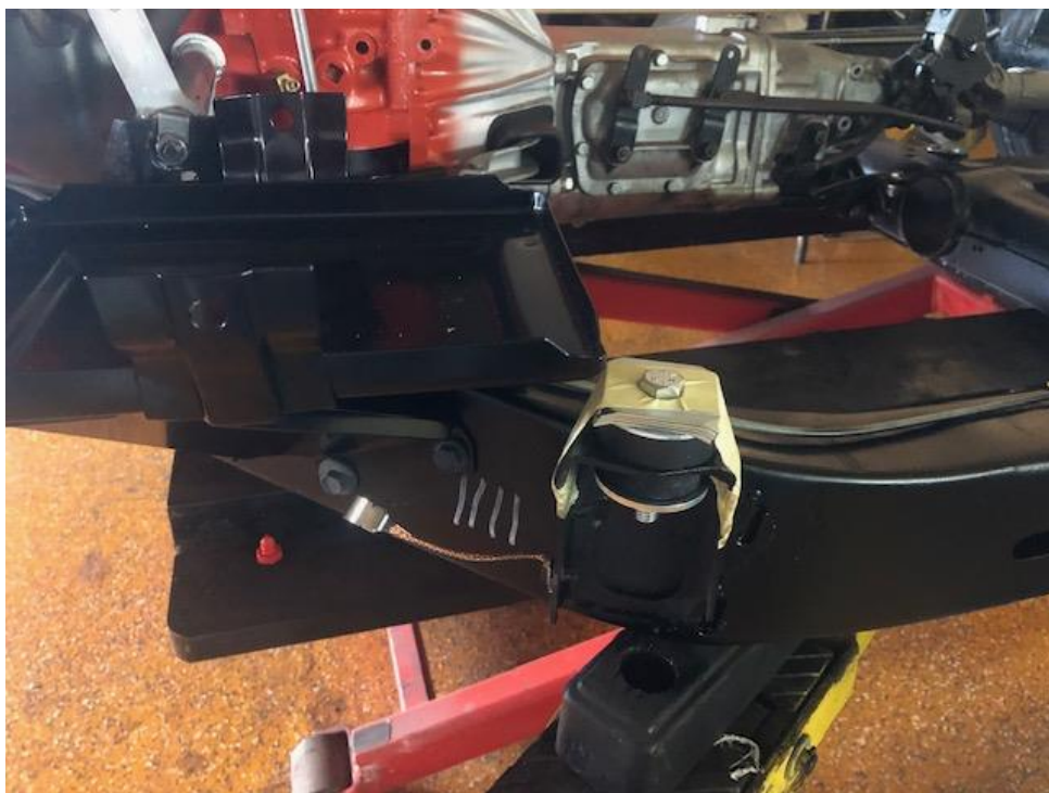
Front drivers side mount 4 shims used along with the tape and earth connections.
