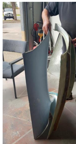
Fender panel being removed from the mould
