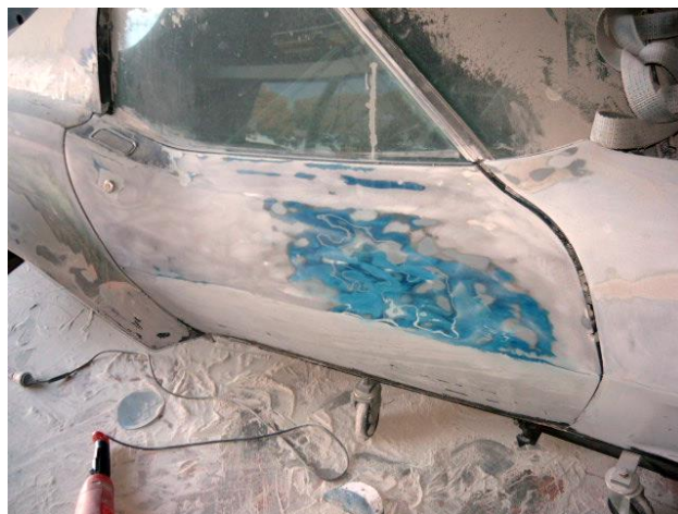
Paint removal and note top of front fender coming away from the birdcage.
