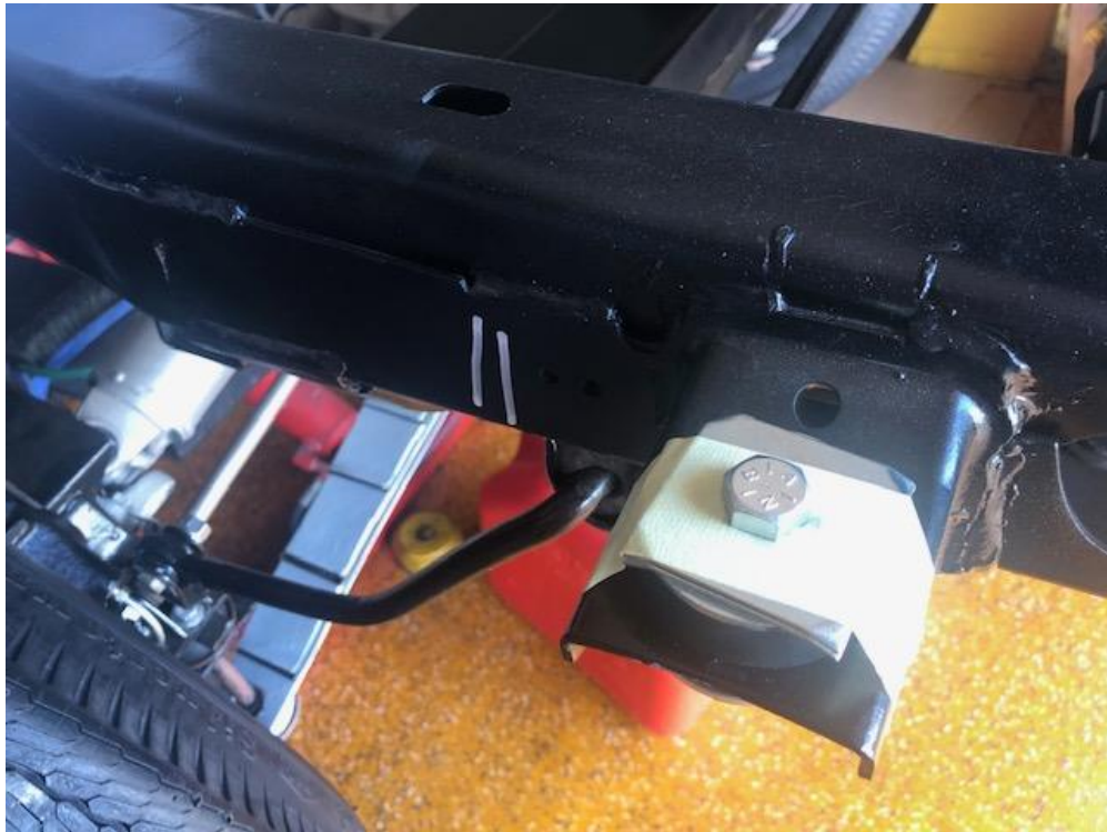
Rear Drivers side mount 2 shims used
