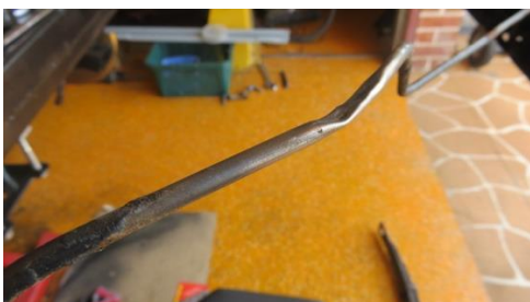
Flattened crossover brake line
