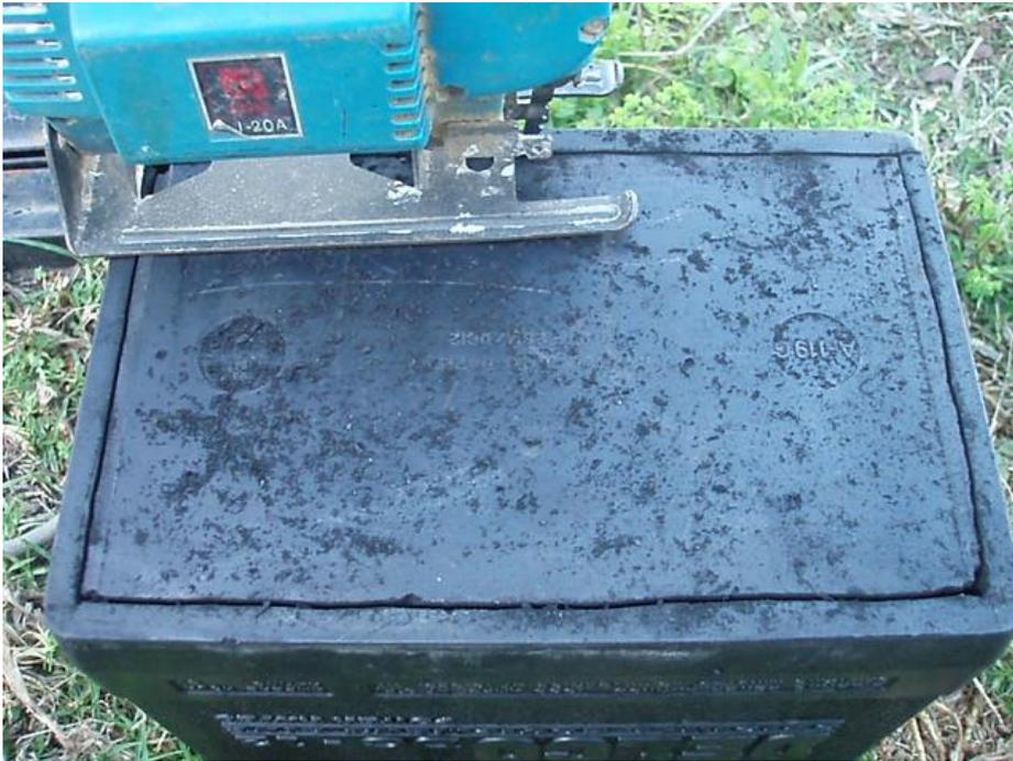
After completing this process, I was able to remove the second section to expose the lead plates and their insulating dividers as shown in the next photos.
