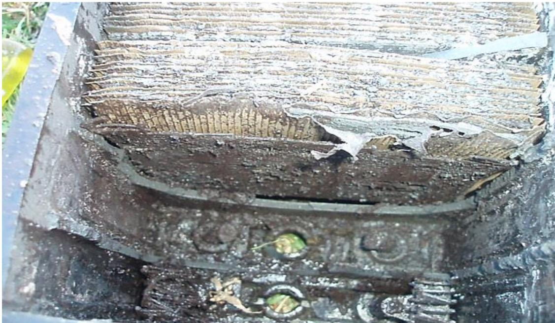
With a sharp wood chisel, I was able to remove the two side dividers, exposing the next set of plates. Now I have more room I can remove the plates one by one till I have that section is cleared. All I had to do is disconnect the plate from the terminal at the top, so it would come out in one section, working forward until there are no more sections left, as shown in the next photo
