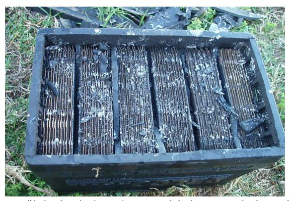
This process did take a long time because it was extremely hard to remove as the plates would break up easily. After a while I was able to have a clear cavity in the battery. As shown in the next photo;
