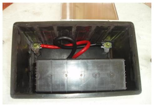
The next thing to do is install the base into the old unit covering up the new battery inside. Turn the battery over and install the newly painted caps with AC DELCO in yellow paint I used foam to space the new battery away from the edge of the old case, restricting its movements.
