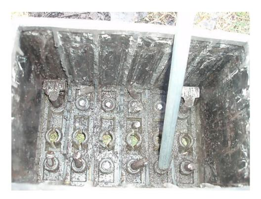
The next thing to do is clean out all the connection points from each cell to the bridging bar at the top of the battery, leaving the two connectors on the bottom side of the Positive & Negative posts. I was able to remove the connection points by using a piece of tube to snap the pins off at their base, as shown in the photo above;
