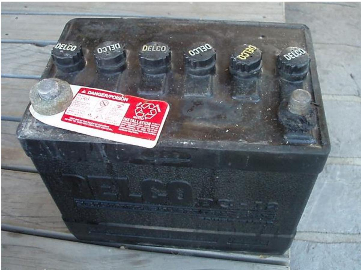
The decision was made to remove the complete inside out of the battery and install another battery inside, because the case was in good condition.
