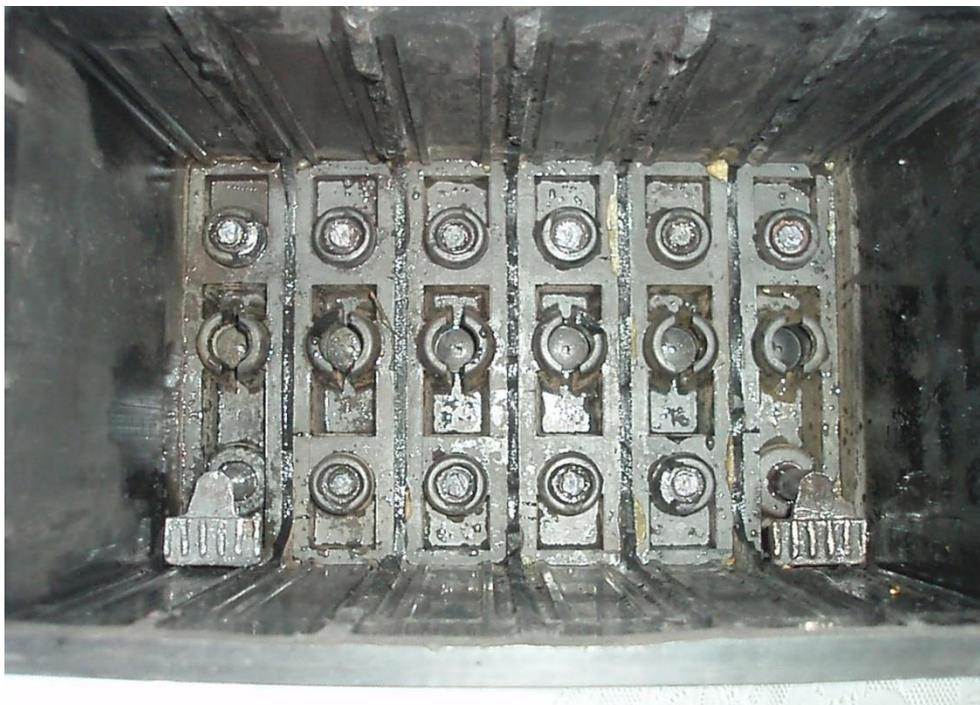
I then cut a piece of 3mm flat rubber sheet to cover these broken old terminals using Silastic to hold it in place. This will ensure the new battery doesn't short anything out.
