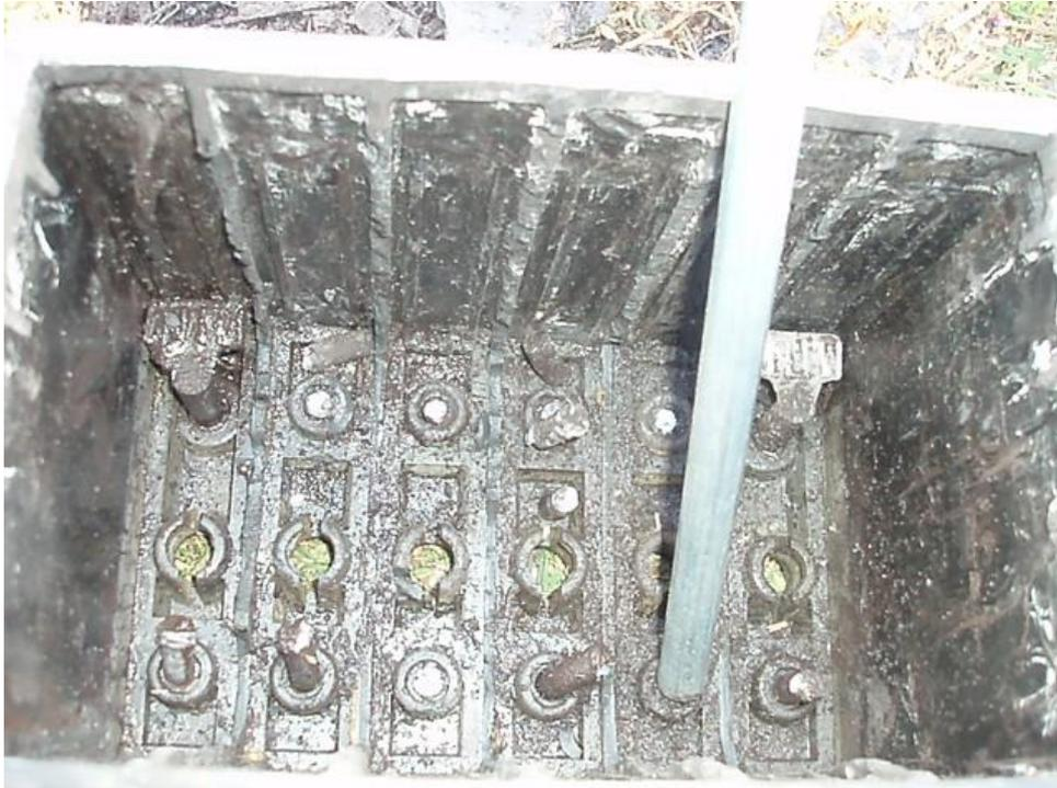
The next thing to do is clean out all the connection points from each cell to the bridging bar at the top of the battery, leaving the two connectors on the bottom side of the Positive & Negative posts. I was able to remove the connection points by using a piece of tube to snap the pins off at their base, as shown in the photo above;
