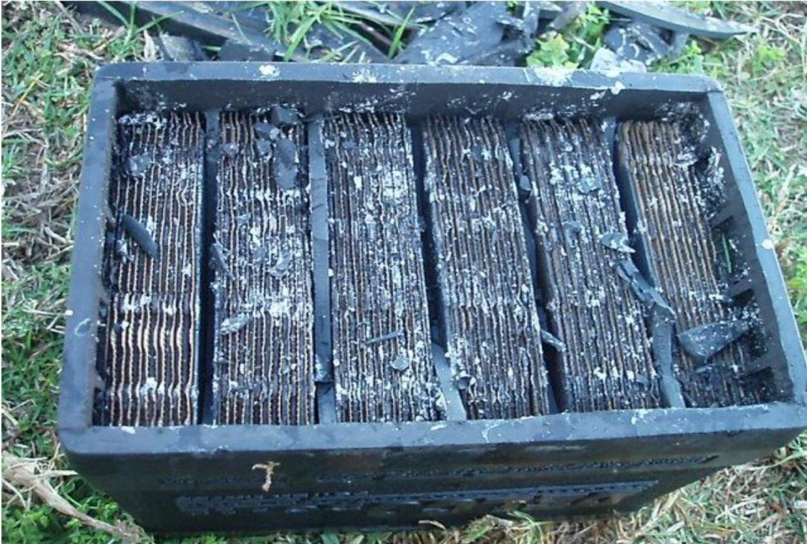
This process did take a long time because it was extremely hard to remove as the plates would break up easily. After a while I was able to have a clear cavity in the battery. As shown in the next photo;
