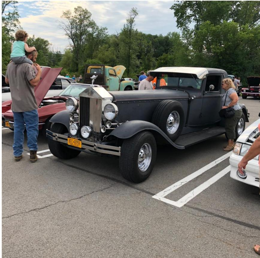
32 Ford body with a Straight 8 engine with a Rolls Grill
