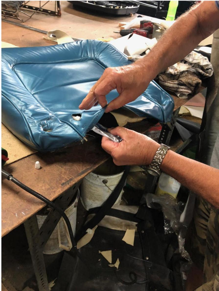
He removed the cover off the foam and glued a mesh “back” to the underside of the seat cover.
