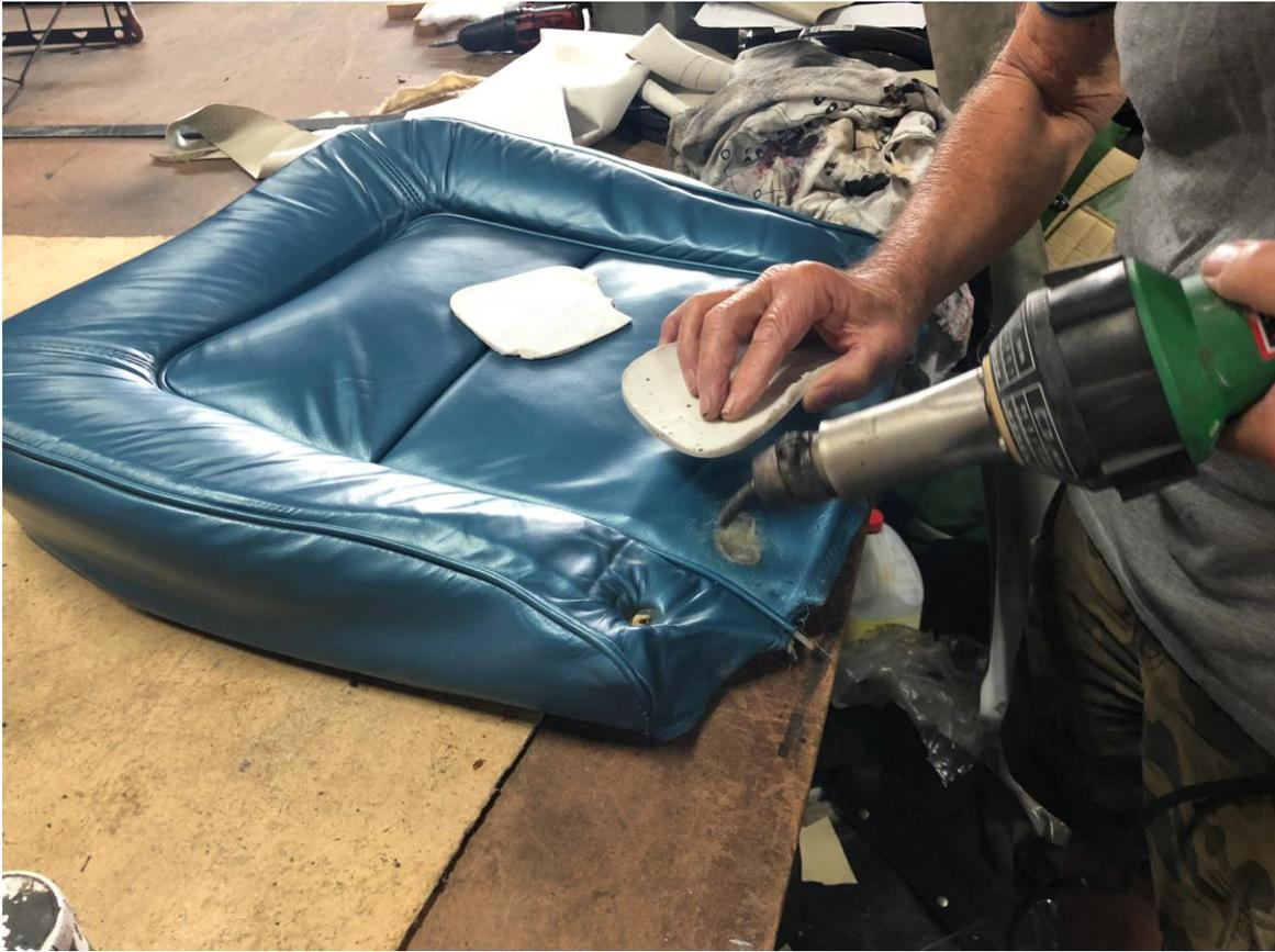
He did this process twice and then a third covering of just the straight vinyl paste. Just before he set it with the heat gun, he pressed a piece of leather into it to give it a leather grain and then set it with the heat gun.
