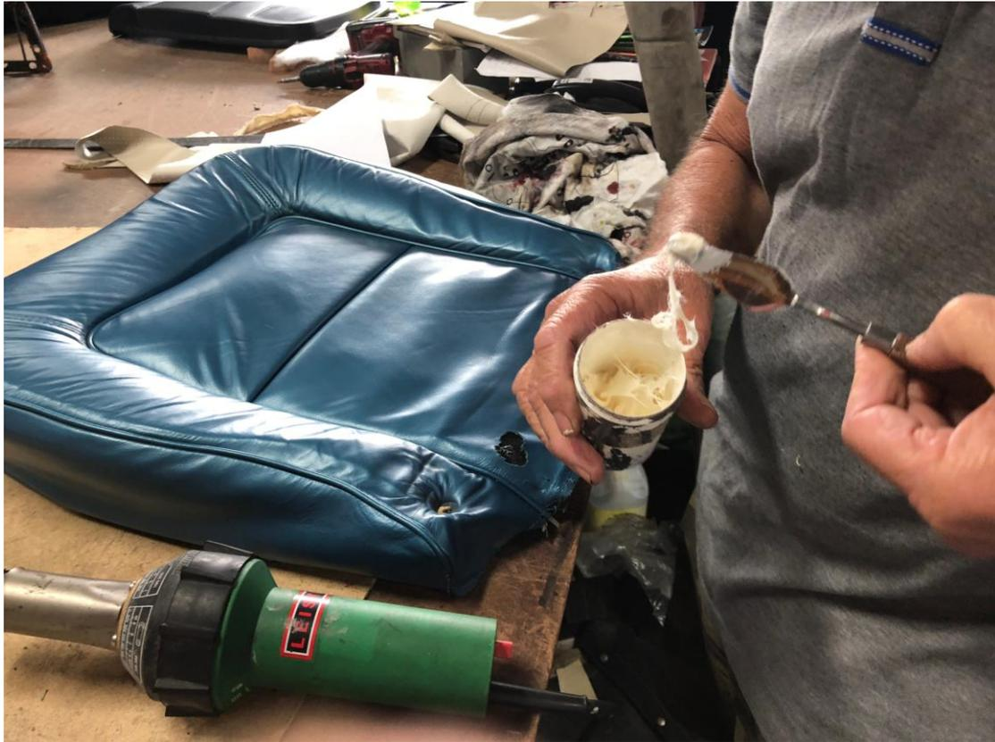
He then, with a spatula, applied vinyl paste with a fibrous filling in it, then, used the heat gun to set it.
