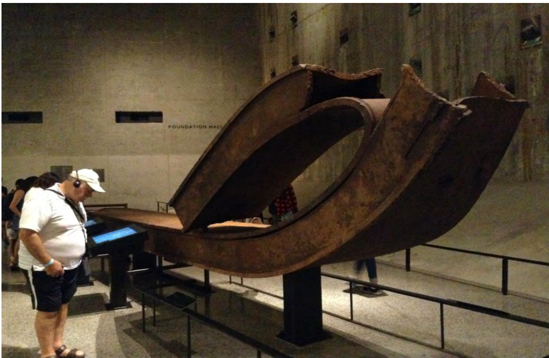
The force of the collapse of the building bent this column.
