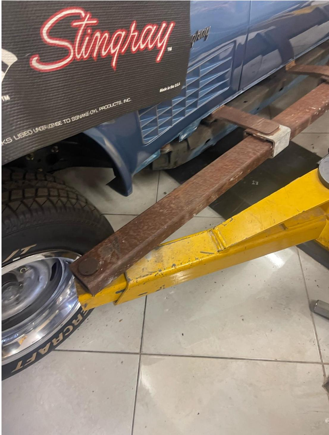
The system I use with my 2-post hoist, is I made up this 150 x 50mm RHS and located 50mm steel pins through it, into the holes on the hoist frame to support the RHS. I then made sliders that can be poisoned anywhere on the RHS with a 12mm x 200mm Welded to them, I then have a 90 deg, by 60mm turnup. This then can make contact with the bottom of the birdcage, so we are lifting the whole car by the bird-cage.
