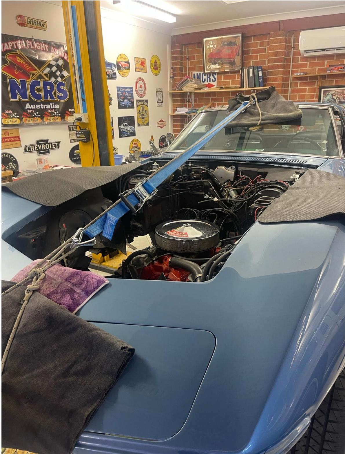
The main problem we have is the amount of overhang on the front end which is unsupported once it is off the chassis. Bill said he had seen this system used before so we thought we would give it a go. Normally I would be putting the body onto my dolly, but in this case, we intend to leave it on the hoist. As I need to park one of my cars under the body.
