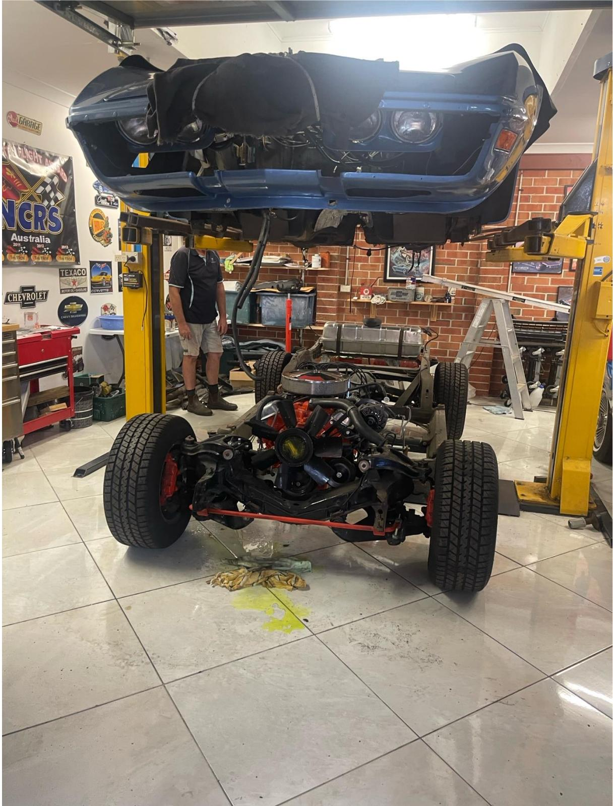
With having so many pairs of eyes, while lifting the body off the chassis was awesome. That we could cover all areas at the same time, checking out if we had missed things that needed to be disconnected. Needless to say, there was one little earth-strap on the aerial, but it was soon picked up
